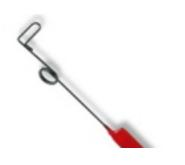
Feather Touch Tension Tool Feather Touch turning wrench with coiled spring head applies pressure from a fraction of an ounce up to 4 oz. Tension wrenches called "Feather Touch" wrenches, are coiled into a spring at the bend in the "L", which helps the user apply constant torque. Some users, however, maintain that such wrenches reduce torque control and the feedback available to the user.
