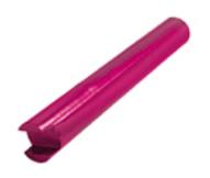
Follower-Small Pin & Peanut Used for most small pin tumbler rekeying jobs. Uses include Corbin small pin, Eagle small pin, Yale small pin and Ilco "peanut" cylinders and others. Diameter = .395 If you're in need of a follower that's a bit larger try the <a href="Large Oversize Follower">Large Oversize Follower</a> with a Diameter of .555
